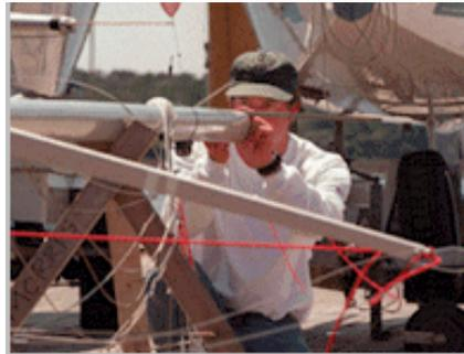
If your spreaders don't already have a mark put a jib trim mark on the spreaders 457 mm (18") out from the side of the mast. I use a felt tip pen or tape to put a 1" band around the spreader. In winds under 18 knots the jib leech will line up with this mark. In more wind it will be slightly outside.
